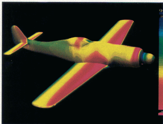
Figure 11 Pressure distribution calculated on the Fw 190 D-9.
