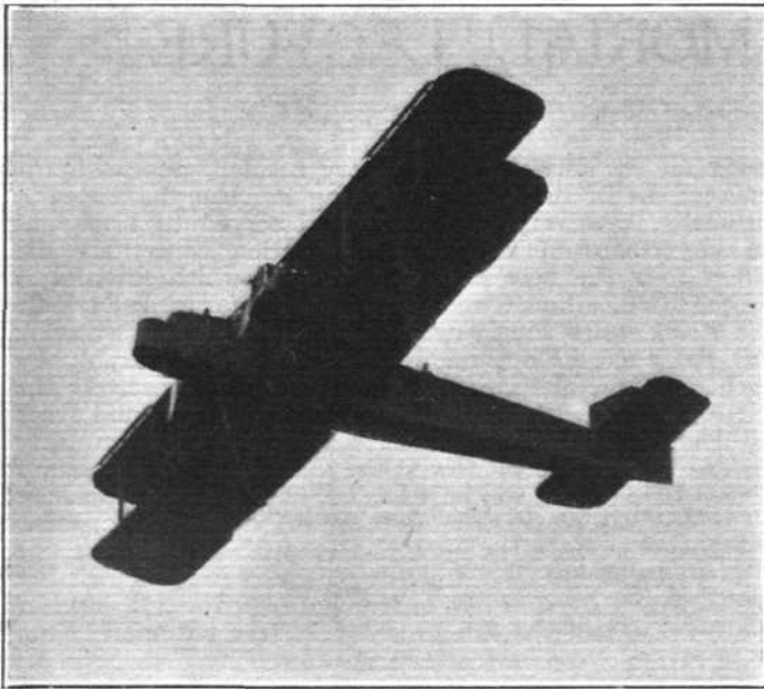
[“FLIGHT” Photograph SLOTS AND THE SERVICE: A Handley Page “Hyderabad” in Flight. Note the automatic slots open at the upper wing tips.
