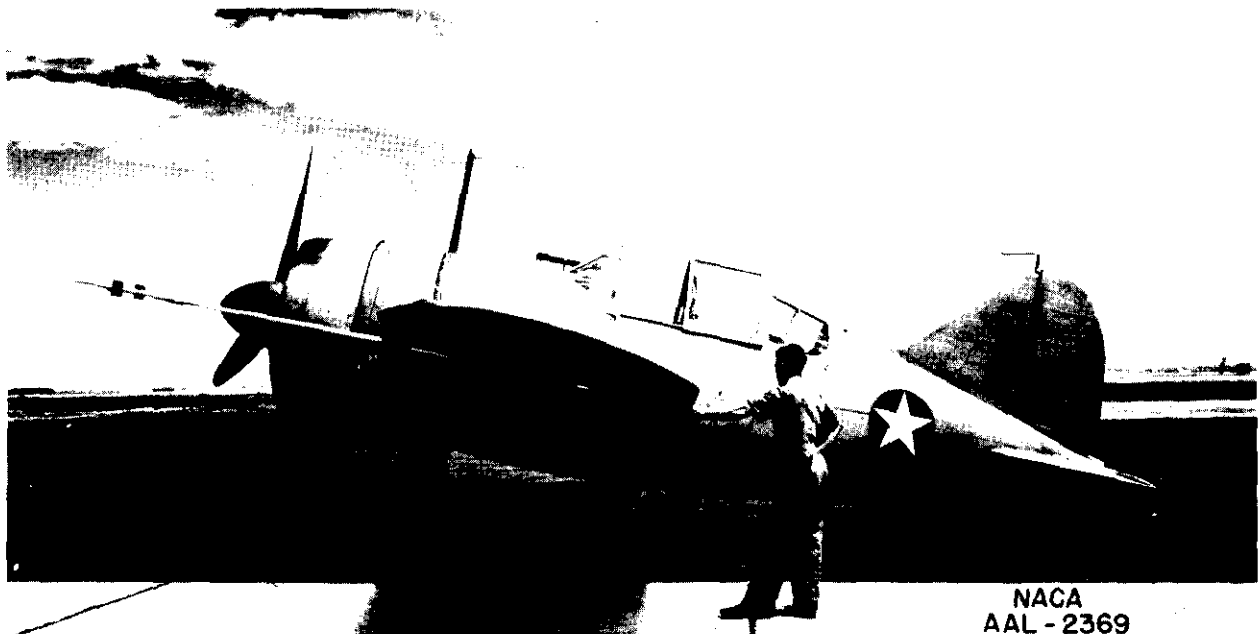
Figure 3.- Side view of Navy F2A-3 airplane as instrumented for tests, flaps down.
